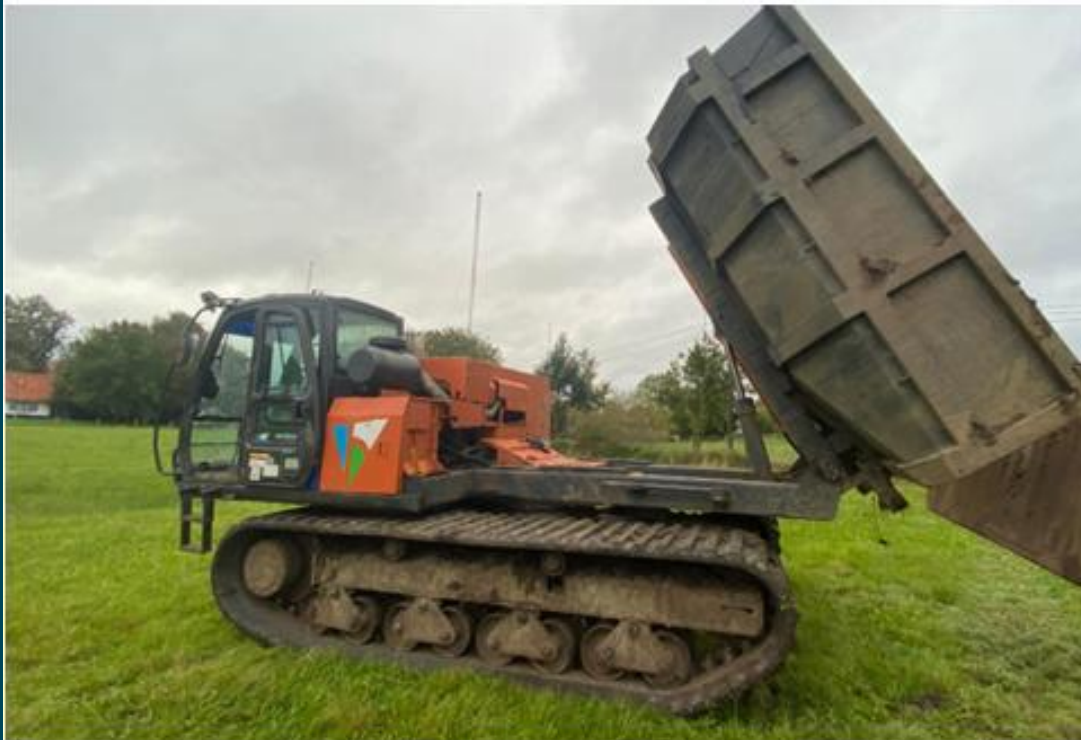
Roterend type rupsdumper
